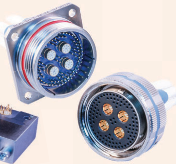
El Ocho® high-speed octaxial contacts with Series 806 Mil-Aero micro miniature circular and Series 792 rectangular packaging
