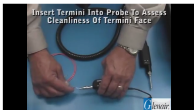
Fiber Optic Terminus Cleaning and Testing - Step 6
