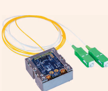
RF-over-fiber low-noise PCB-mount transceiver
