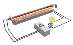
Cables are qualified according to their resistance to fire and other combined parameters, such as mechanical shocks and water spray. These tests are carried out on cables under electrical load.
