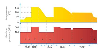
The figure shows the LOCA curve used for the French PWR.
