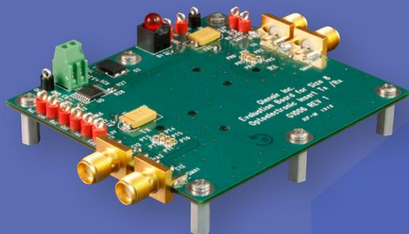
Optoelectronic contact evaluation boards are available for all size #8 transmitters or receivers
