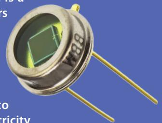
for use as power. When sunlight strikes the PV cell, it is absorbed within specially formulated “semiconductor” material. In the process, the absorbed energy knocks electrons loose, allowing them to flow freely as electrical current. In fiber optic interconnect datalinks, the role of the photovoltaic cell is performed by a miniature photodiode, an optical detector that converts photons into electrons by a process called “quantum absorption,” originally documented by Albert Einstein.
