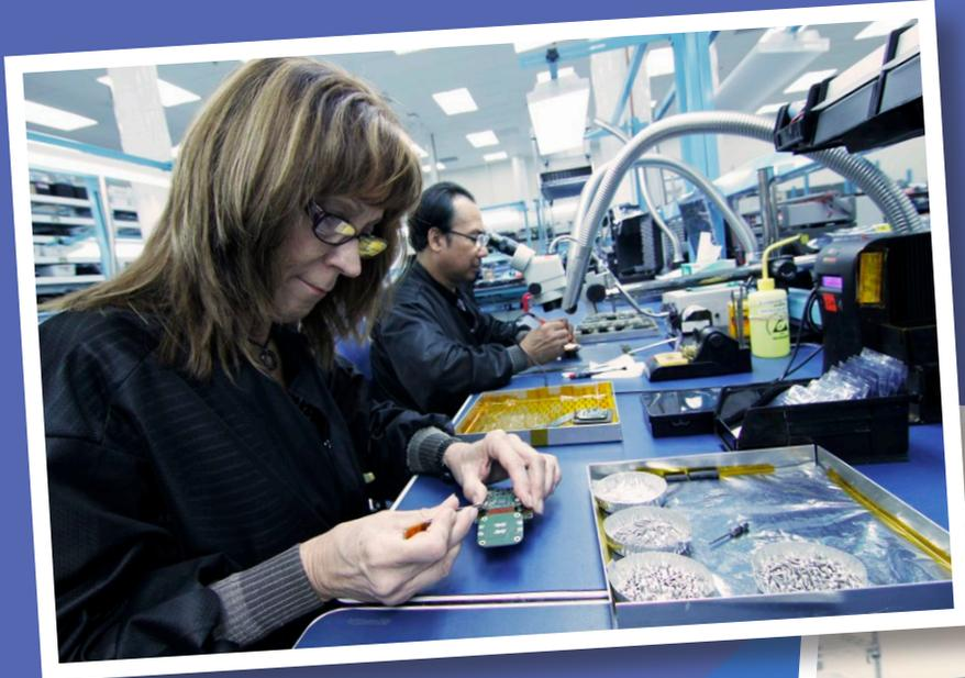
▲ Assembly of ruggedized Ethernet copper-to-fiber media converter subassembly
