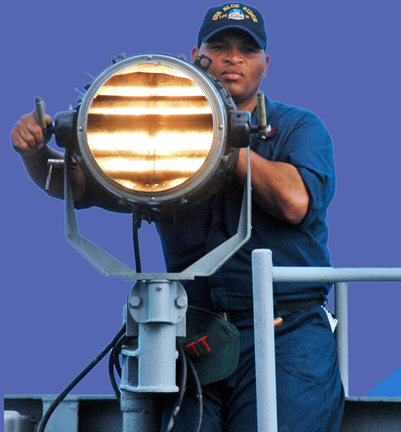
The conversion of electrical energy to visible optical energy is really not so grand of a thing. Folks have been doing it for years. A common light bulb, for example, performs this conversion with the simple flip of a switch. Incandescent light bulbs, such as the one shown here, use a thin filament of tungsten wire to manage the conversion. The current flowing through the wire generates heat, some of which is emitted in the form of visible light.
