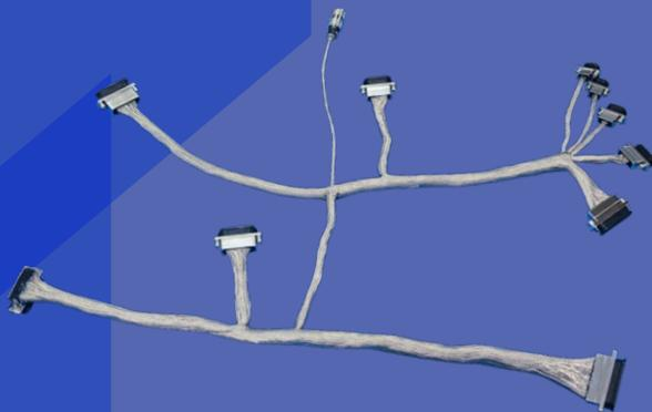
Multibranch Micro-D / Mighty Mouse cable assembly with ArmorLite<sup>™</sup> lightweight EMI shield overbraiding
