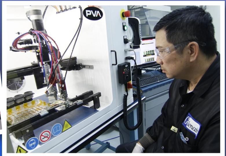
▲ Conformal coating of optoelectronic subassembly
