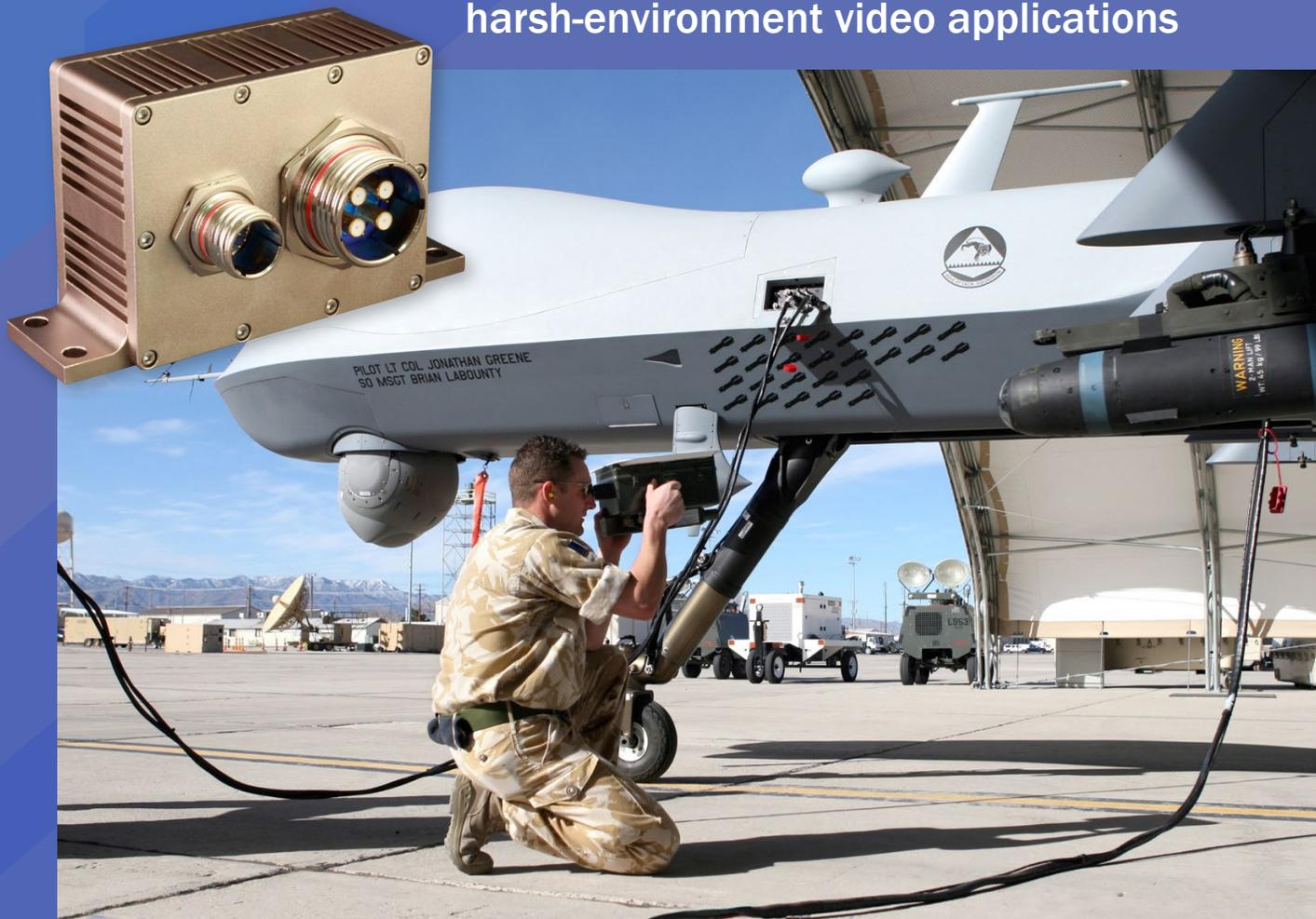
Glenair Copper-to-Fiber-Optic Video Media Converters enable extended link distances, improved EMI and security in harsh environments and provide solutions for both MMF and SMF applications. These media converters support ruggedized military systems applications and are tailored to support a variety of Video protocols including DVI, HDMI, SMPTE (SDI, HD-SDI and 3G-SDI), ARINC 818 and more.
