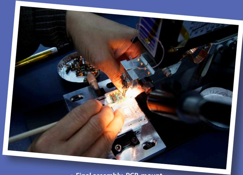
▲ Final assembly, PCB-mount optoelectronic transceiver
