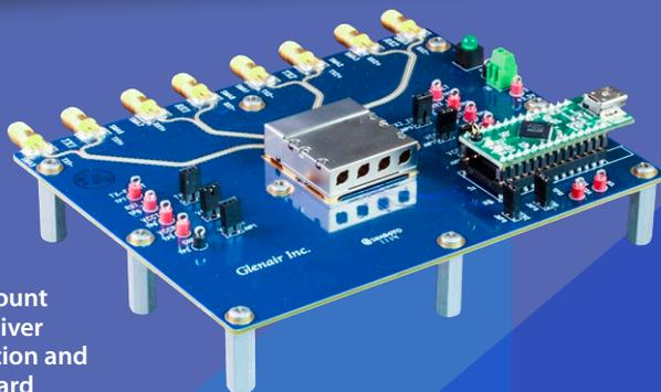
▶ PCB-mount transceiver evaluation and test board
