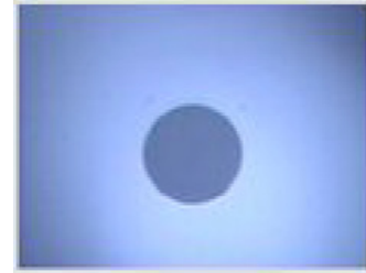
Connector end face after cleaning
