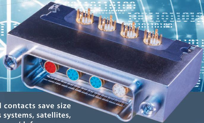
High speed, harsh environment El Ochito® octaxial contacts save size and weight. Suitable for aircraft avionics, weapons systems, satellites, radars, communications equipment and other aerospace/defense gear, El Ochito® contacts are optimized for drop-in use in all connector packages with keyed size #8 contact cavities, including MIL-DTL-38999, ARINC 600, Series 80 Mighty Mouse, Series 791 Micro-Crimp, and others.
