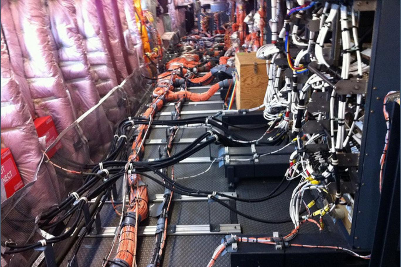
Innovative solutions to EWIS environmental sealing, wire management, strain relief, and EMC shield termination
