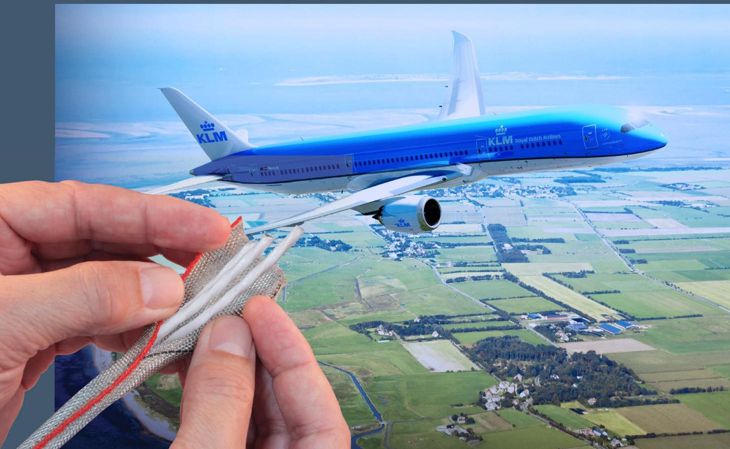
**T**ubular braided sleeving meets the broad range of EMC shielding and mechanical protection requirements of aircraft harness assemblies. But the need to apply shielding materials over already-installed aircraft wire and cable bundles requires new technology. Legacy self-wrapping cable braid has long been available for EMI/RFI applications and abrasion protection, albeit with poor performance due to its heavy weight, inflexibility, and “windowing,” which results in poor shielding performance.
