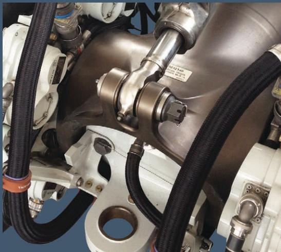
Turnkey wheel well impact-resistant metal-core conduit assembly
