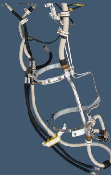
Metal-core conduit wire protection aircraft brake assembly
