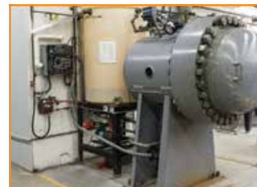
Hydrostatic test chamber
