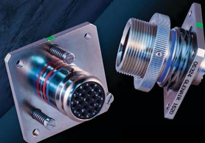
**Assisted separation force:** Adjustable kick-off style with spring-loaded posts and an adjustment ring to calibrate separation force. A second style uses wave springs on the shell body.
