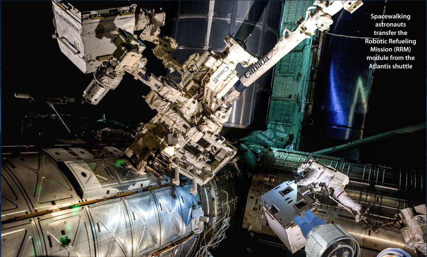
Spacewalking astronauts transfer the Robotic Refueling Mission (RRM) module from the Atlantis shuttle
