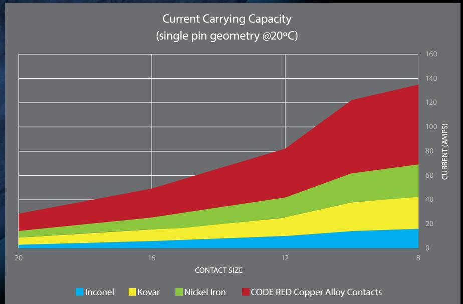
**APPLICATION NOTES:** CODE RED is a viable drop-in solution for conventional glass-to-metal seal hermetic connectors with the following exceptions:
