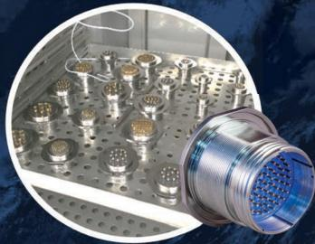
Connectors utilizing CODE RED hermetic encapsulant sealing went through a grueling qualification test and validation process to prove material durability and hermeticity. Validation testing including 100 cycles of thermal shock IAW EIA-364-32 Test Condition A -65°C to +200°C while maintaining hermeticity followed by 1000 hours of thermal aging at 200°C. Additional tests included:
