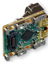
PCB-mount opto-electronics feature Samtec high-speed surface-mount connectors
