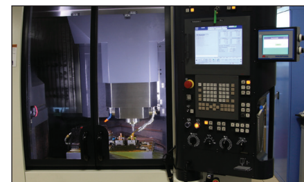
High speed and high precision milling machine for tools and machine building
