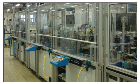
High speed switch assembly machine designed and built by C&K
